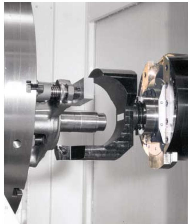
**Turning, drilling and milling by means of DBF spindle head**
